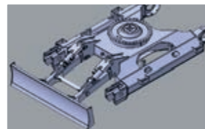
Dozer blade (on DX225LC-3) For dozing and working on sloped terrains. It also increases stability when lifting.
